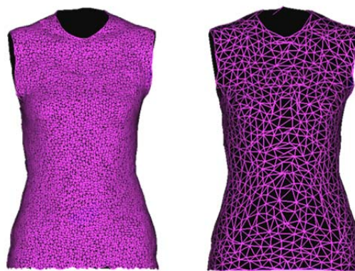
Fig. 1. The polygon data of a subject after cutting off the unnecessary area for analysis (left) and Homologous model of the same subject (right.)
