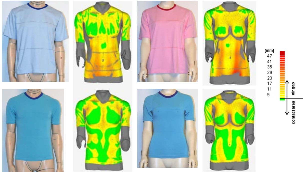
Figure 2. Photographs and corresponding post-processed exemplary 3D scans indicating the contact area and the air gap thickness of the loose- and tight-fitting garments in male and female manikins.
