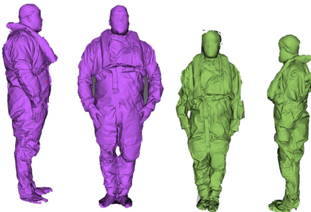
Figure 9. Illustrating the difference in snugness of fit between a large and small individual.
