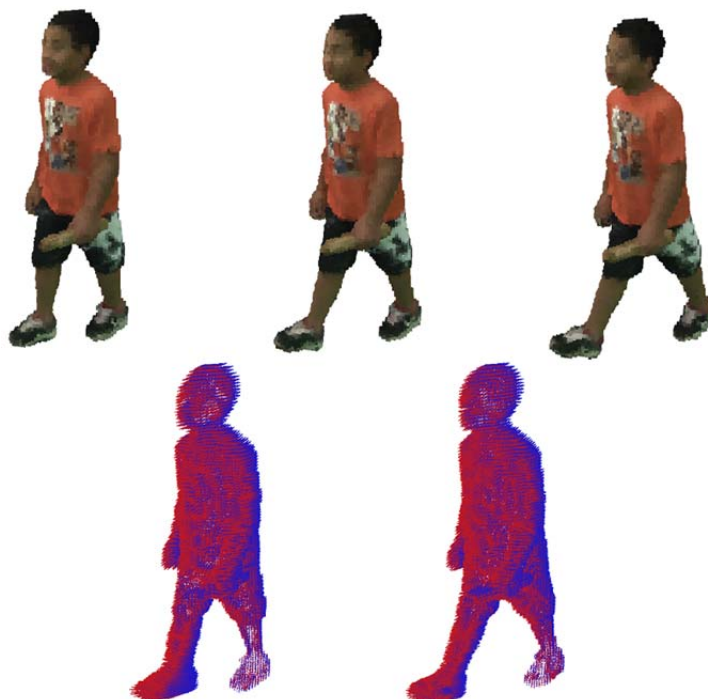
Figure 8. Model tracking results for "Kevin" rush Top: three successive frames of the volumes sequence. Bottom: two intermediate motions flows.
