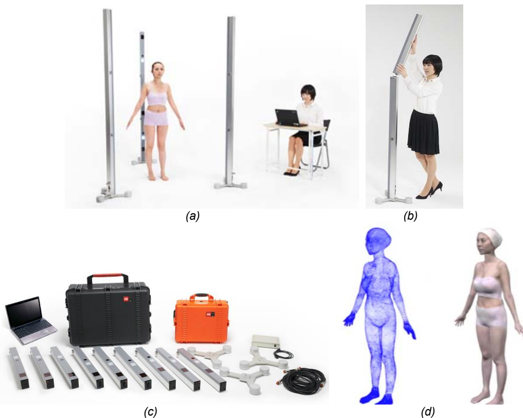
Fig. 1: New traveling type 3D full body scanner. (a) During scanning. (b) Each tower can be disassembled into three modules. (c) All components. (d) The example of interpolated data. (Point cloud / Closed surface with texture)
