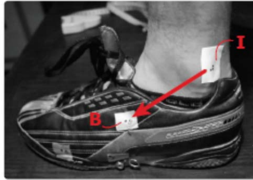
Fig. 7. Markers I and B on the lateral side of the leg and foot.
