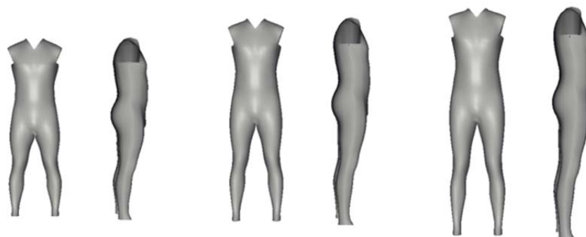
Fig. 7. Changes in the 1 st PC for the male body model. Left: -2 \times \text{Standard Deviation (SD)} , middle: 0 \text{ SD} , right: +2 \text{SD} .
