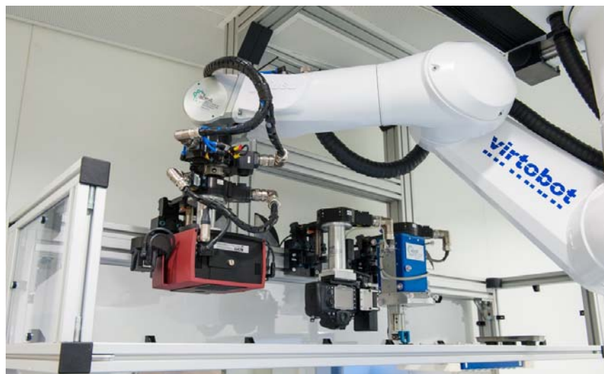
Fig. 2. Tool stand during automatic tool change. Left to right: Surface scanner, digital photo camera for photogrammetry and biopsy module.
