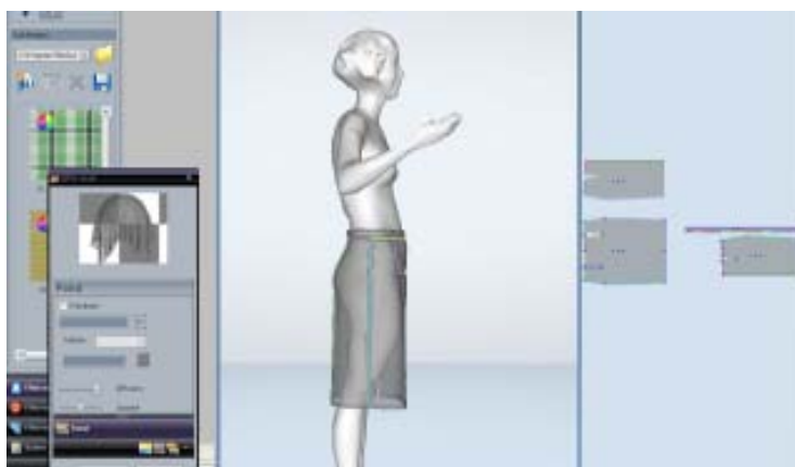
Fig. 6. 3D simulation of a skirt pattern (straight part) on an avatar of a scanned person (source: Lectra)
