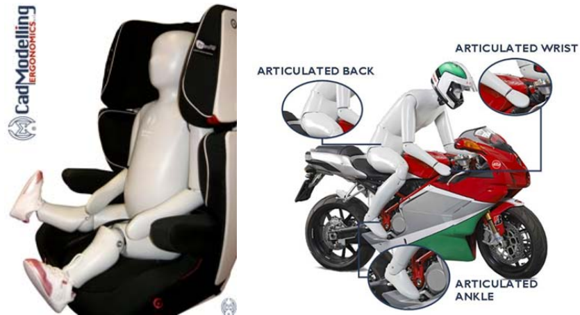
Fig.13 . "Active and SuperActive FORMAX® for ergonomic and safety tests".
