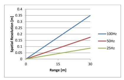
Fig. 2. The spatial resolution of SICK LMS-511 at 100, 50, and 25Hz.
