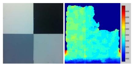
Fig. 6. Left, a flat plate with four fields with different reflectivity and on the right a Kinect depth map of the plate at 5.5 m. The Kinect has obvious problems with low reflecting targets.
