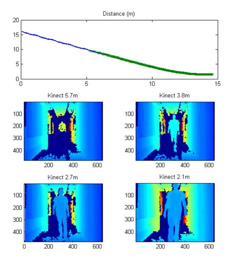
Fig. 7 Top, distance to target as function of time, blue is LMS-511 data and green is Kinect data. Below, 4 depth maps from the Kinect at 5.7m, 3.8m, 2.7m, and, 2.1m.
