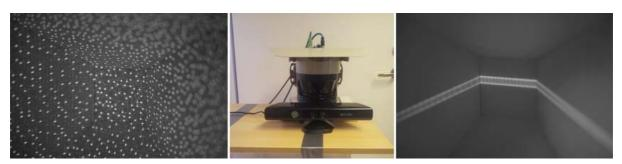
Fig. 1. Left, the IR pattern of Kinect (NIR image). Middle, the Kinect placed in front of the LMS-511. Right, the laser pulse of LMS-511 (NIR image).
