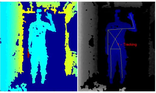
Fig. 3. Left, color coded depth map from Microsoft Kinect. Right, pose tracked with OpenNI.
