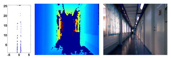
Fig. 5. Left, laser range measurements of the empty corridor. Middle color coded depth map from Microsoft Kinect. Right, the visual image of Microsoft Kinect depth.
