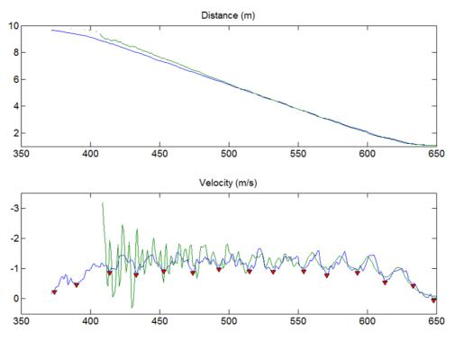
Fig. 9. Upper, distance to target. Lower, target velocity. Green line is Kinect and blue is LMS-511.
