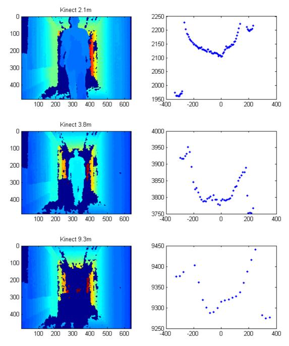
Fig. 8 Left, Kinect depth maps at 2.1m, 3.8m, and, 9.3m. Right, the corresponding LMS-511 measurements at the same distance and time.
