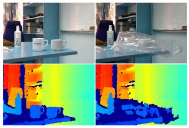
Fig. 7. Top, visual image of mugs without and with surrounding plastic. Bottom, Kinect depth image of the corresponding scenes.
