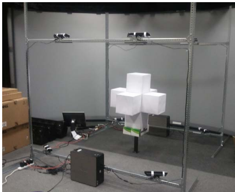
Fig. 1. The multi-Kinect scanner with central calibration object
