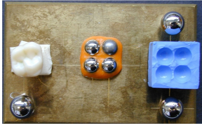
Fig. 12. The simulation model of the molar tooth surface, on the left (white) is a molar tooth surface, and on the right (blue) is an impression of the simulation model.
