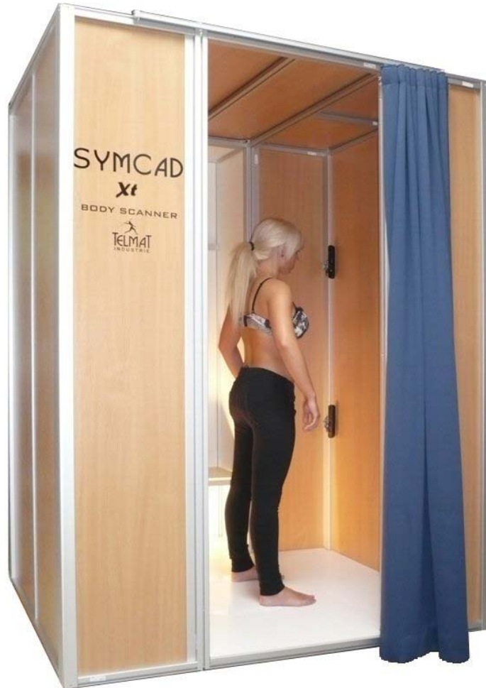
Fig. 5. SYMCAD™ Xt 3D body scanner for retail shops, based on ASUS Xtion® depth sensors.
