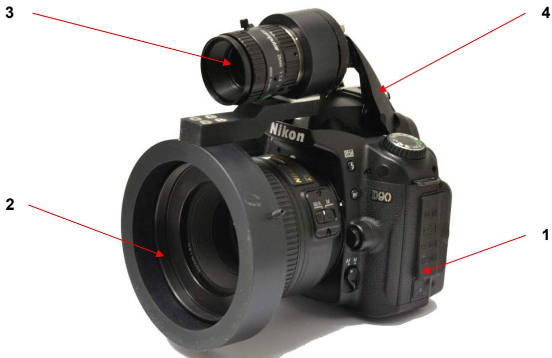
Fig.1. Image of the measuring system. 1) DSLR camera Nikon D90. 2) 50mm fixed focal lens. 3) Grating projection system. 4) Built-in flash.
