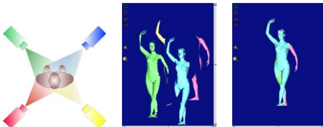
Fig. 3. Combination of different scans in a 3d model by means of calibration.
