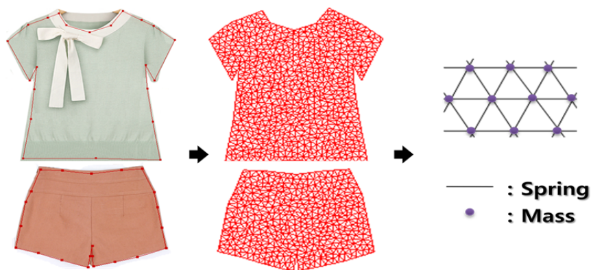
Fig. 2. Mass-spring model for a garment image.
