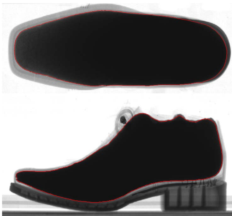
Figure 2: Top and side x-ray images of a shoe filled with a contrast media
