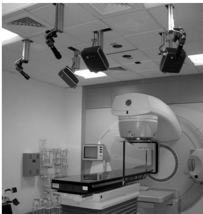
Fig. 1. The three colour channel separated camera-projector pairs of our Fourier profilometry optical surface measurement system in a radiotherapy treatment room at The Christie. The rotating gantry and imaging panels constrain the geometry of the system to the highly non-optimal arrangement pictured. The camera and projector axes have incident angles of approximately 40°.
