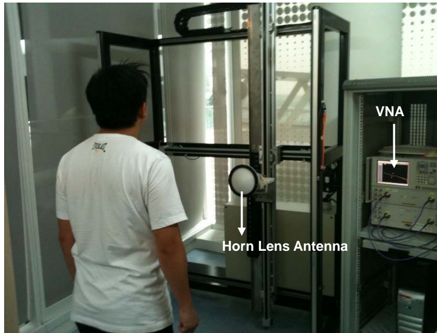
Fig. 1. Overview of the system setup at millimeter wave frequency.
