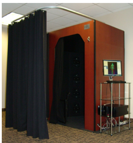
KX-16 Low Cost 3D Body Scan booth using Kinect Sensors
