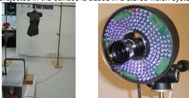
Fig. 3. Acquisition system (left – laser scanner and the female phantom torso; right – one of the cameras from the tracking system).
