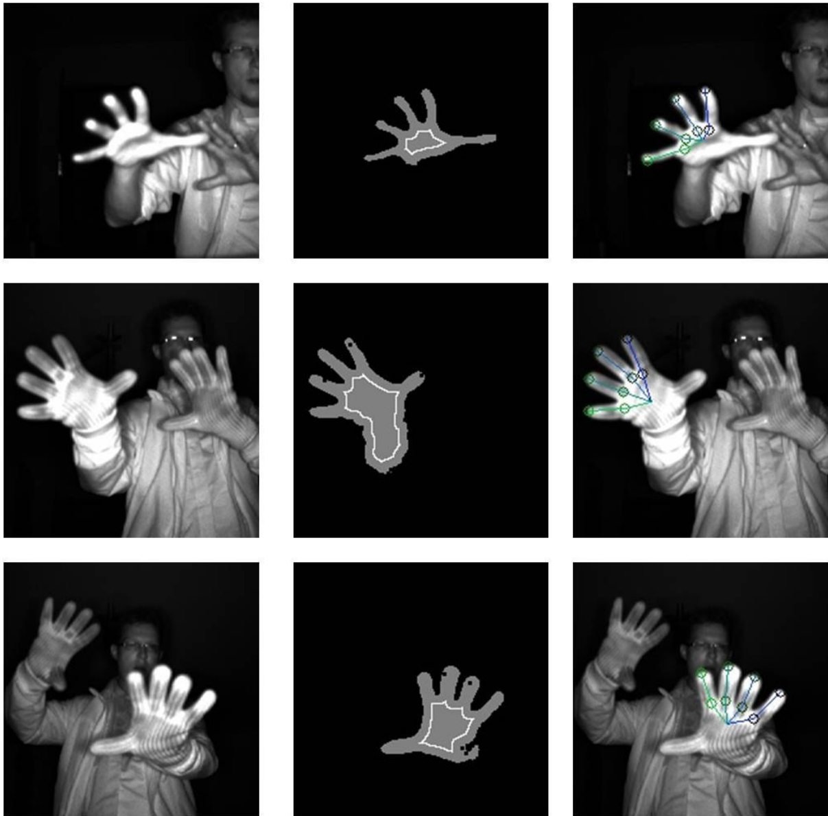
Figure 5: Experimental results. Hand detection of a hand covered by a glove and with sleeves. From left to right each row displays the original amplitude data, the result of the fine segmentation (gray: segmentation; white: palm contour) and the detected finger tips, root finger joints and center of palm. Note that a second hand in the field of view does not disturb the hand analysis, since the processing pipeline was designed to analyze only the hand which is closest to the ToF camera.
