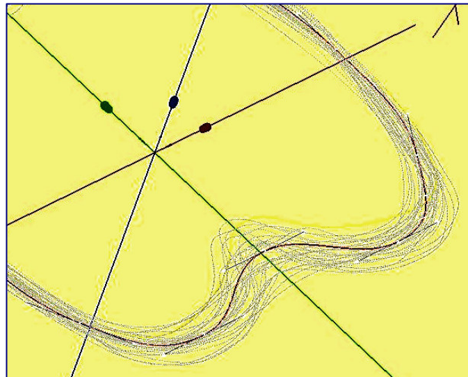
Fig. 6: Determination of spline curves, describing a statistically well-founded curvature for standard table sizes from measured data (measurement see [7])
