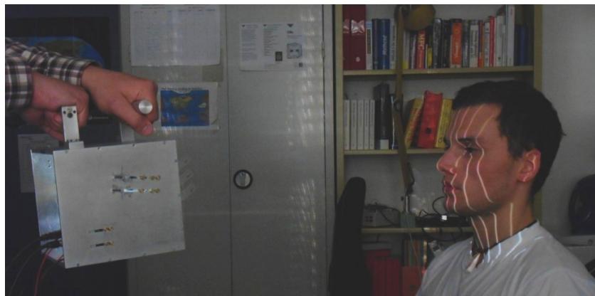
Fig. 4. The realized sensor for a full 360^\circ 3D acquisition of a person's head. Depicted is the sensor "in action". The sensor is freely hand guided around the object while capturing 3D data "on the fly".
