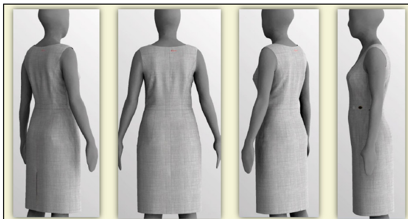
Fig. 14: 3D simulation on a realistic Scanatar representing the German ladies standard size 38
