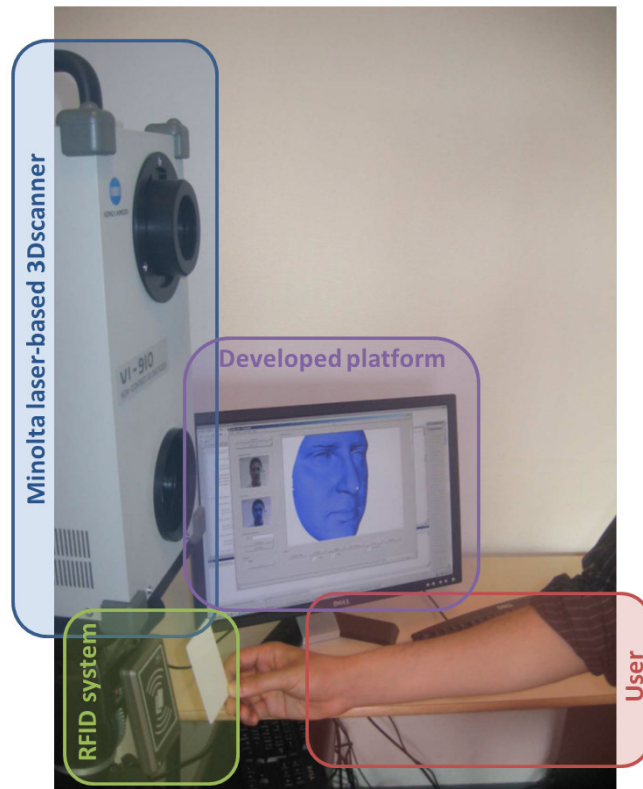
Fig. 2. The developed platform (software) in his testing environment (laboratory conditions).
