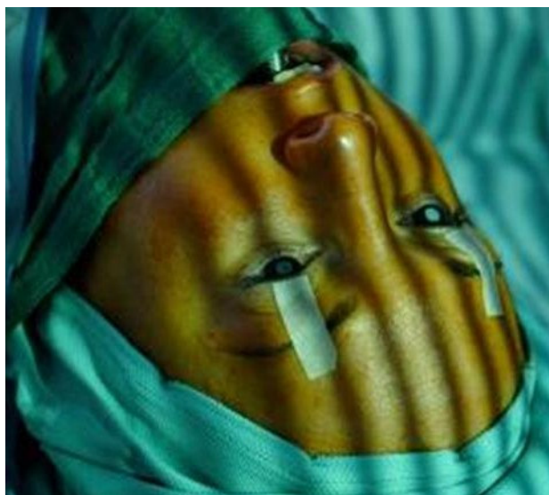
Fig. 2. Patient wearing special contact lenses to capture the 3D-positions of both eye pupils.
