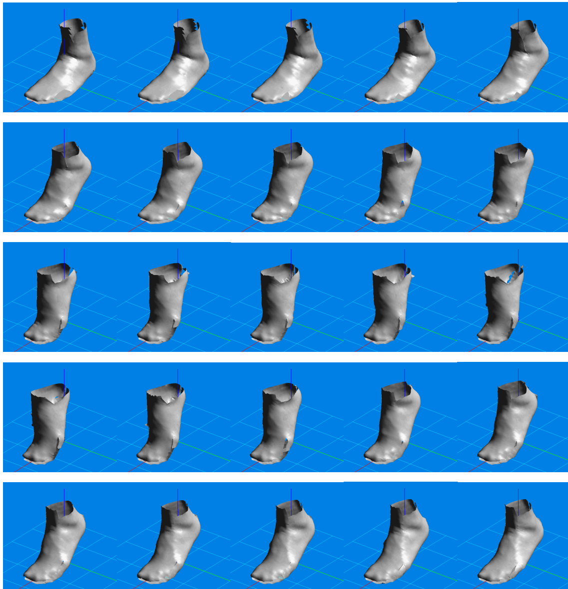
Figure 5: Three-dimensional foot shape acquired while the person is stepping up on their toes.
