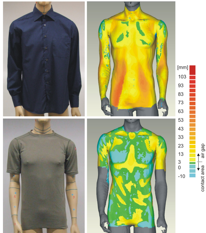
Fig. 3. Photographs and the view of post-processed 3D scans indicating the contact area (blue and green) and the air gap thickness (colour scale from yellow to red) of the shirt and the T-shirt.
