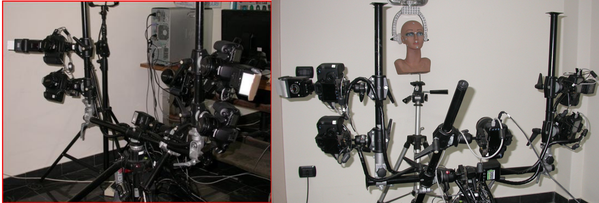
Fig. 5 Photogrammetric set-up with target on the background and applied on the face, using 5 cameras.
