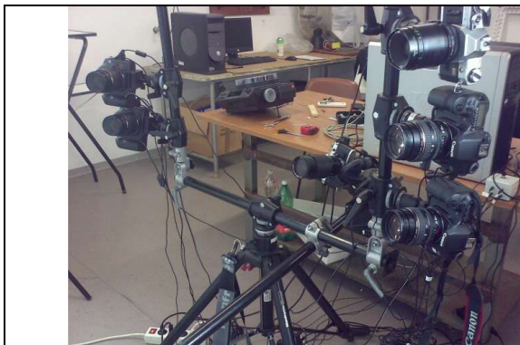
Fig. 3. 4-Camera photogrammetric system set-up
