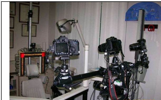
Fig. 1. photogrammetric set-up system with 3 cameras, projected grids and targets in a dark environment
