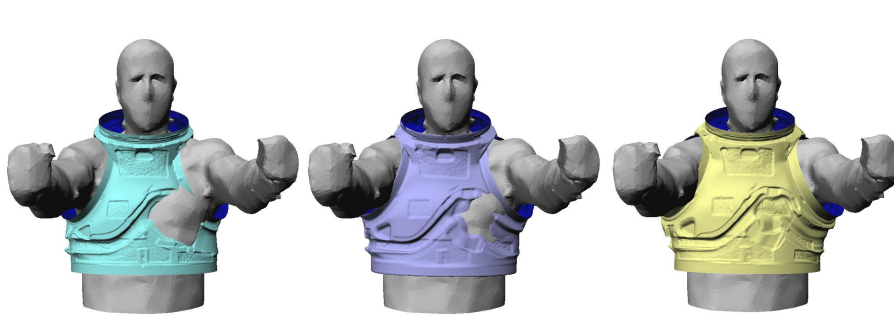
Fig. 4. Hard Upper Torsos overlaid onto a scanned subject: Medium (left), Large (middle), and X-Large (right).
